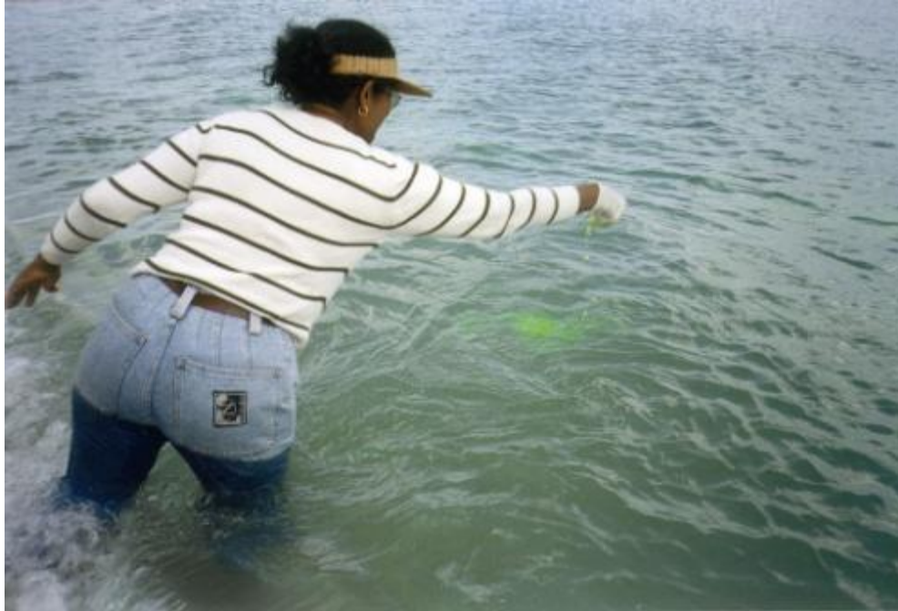
Measuring longshore currents with fluorescent dye.
