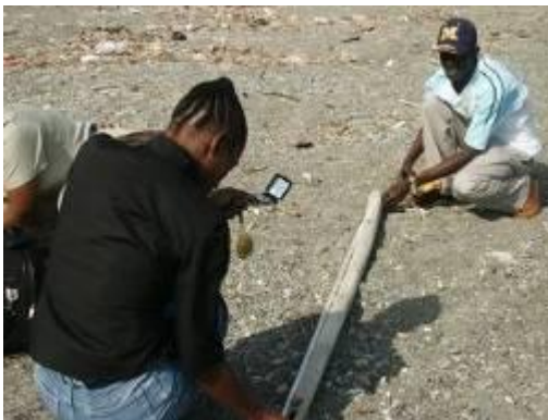
Making a wave pole from a piece of bamboo found on the beach, Jamaica
