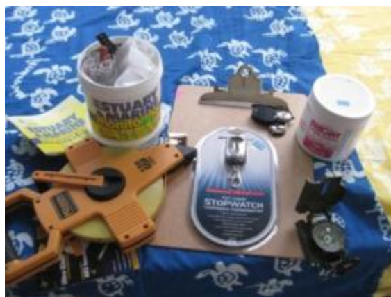
Sandwatch equipment including (from left going clockwise) tape measure, water quality kit, clipboard, hand lens, dye tablets, compass, stopwatch.
